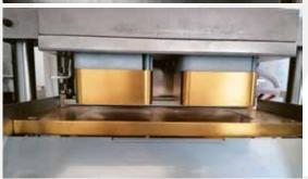
The material used for the forming mould is the tempered steel, coated with titanium nitride (TIN or Tinite), in order to ensure a long life and to reduce fouling during production. The moulds, as all the other parts which are in contact with food, are realized with food-grade certified materials.
