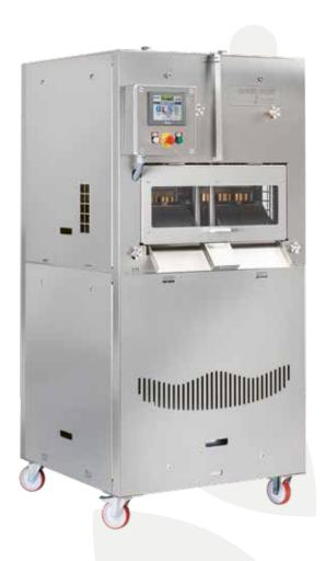
Green Puff is composed by 2 independent presses, powered by compressed air and electricity, which are placed on a structure with pivoting wheels and a drawer in the lower part to collect production waste.
