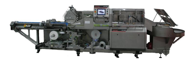
Redpack's NTS-BMI has a unique V-shape infeed that serves to stabilise the product and prevent it from rolling around; something that is especially critical while running at high wrapping speeds and on unstable field rigs. There is also an overhead paddle system that holds the product across the transfer point to ensure accurate product placement onto the film.
