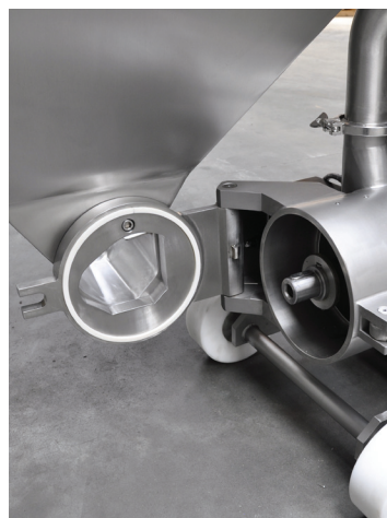
Separated hopper from motor shaft
