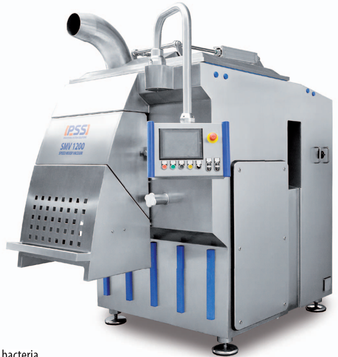
PSS SMV – speed mixer SM with vacuum system
