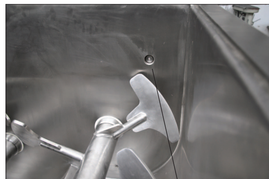
Dosing hole for water dosing
