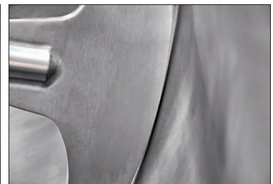
The minimum space between the mixing paddles and the hopper wall
