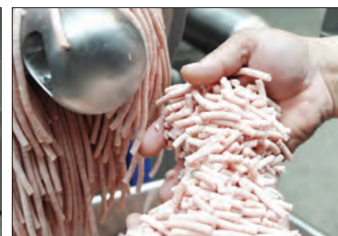
The size of the product after grinding depends on the selected grinding set
