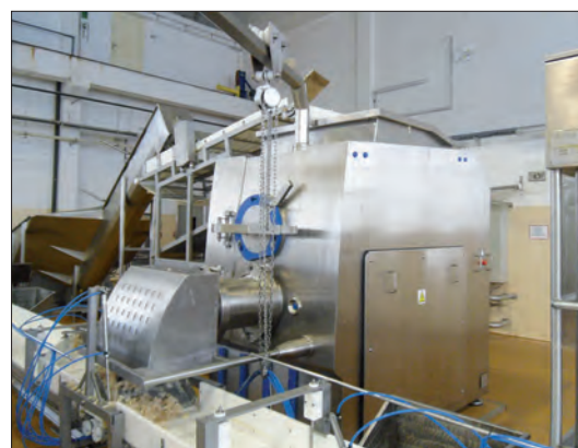
Speed Grinder PSS SCG during cutting skins
