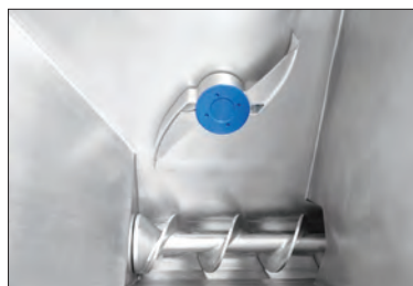
Hopper of SG 200 with feeding wing
