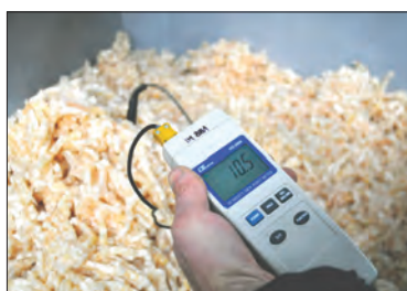
Measuring the temperature of the product after cutting
