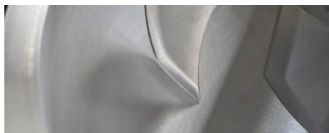
Detail on distance between bowl and knife
