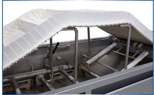
ACCESSIBLE BELT DESIGN FOR EASIER CLEANING
